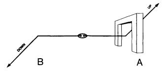
The original two-particle system with zero spin is at the center. One of the particles goes to area A. In area A it goes through a Stern-Gerlach device. In this case, the Stern-Gerlach device gives it a spin *up*. Therefore, we know *without measuring* that the other particle, which has gone to area B, has a spin *down*.
