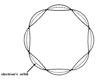
Where the crest of one wave meets the trough of another wave, they cancel each other and the surface of the water along this line of interaction is calm. These calm areas are the nodes which separate the standing waves. In the double-slit experiment, the nodes are the dark bands in the pattern of alternating light and dark areas. The light bands are the crests of the standing waves.
