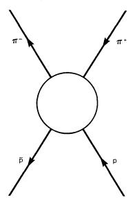
Every time a diagram is rotated it depicts another possible interaction. This particular S-Matrix diagram can be rotated four times. All of the particles that can be depicted by rotating a single element of the S Matrix are intimately related to each other. In fact, all of the particles represented in an S-Matrix diagram (including those discovered by rotating the diagram) are defined in terms of each other. Which of them are "elementary" is a meaningless question.
