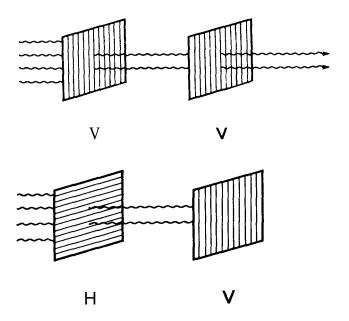
Whenever two polarizers are oriented at right angles to each other they block all light. No matter how the pair is twisted or turned as a unit, as long as they remain at right angles to each other, no light passes through them.
