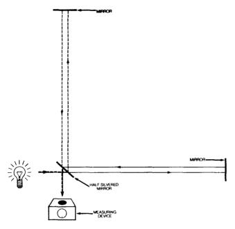
other, and back again The two beams then reunite via the same half-silvered mirror and travel (---->) into a measuring device By **observing** the interference created by these converging beams in the measuring device, any difference in velocity between them can be determined accurately
