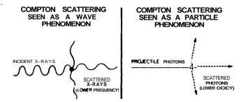
Compton could tell just how much energy the deflected x-rays lost by measuring their frequencies before and after the collision. The frequencies of those x-rays involved in near head-on collisions were noticeably lower after the collision than before it. This meant that they had less energy after the collision than they had before the collision. Compton s x-rays were impacting with electrons exactly the way that billiard balls impact with other billiard balls.
