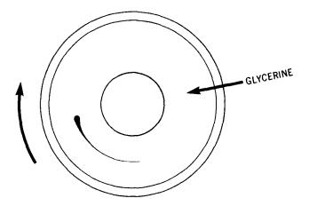
If we begin to rotate one of the cylinders, say in a clockwise direction, the drop of ink spreads out in the opposite direction, making a line which grows thinner and thinner until it disappears altogether. The ink droplet now is enfolded completely into the glycerine, *but it is still there*. When we rotate the cylinder in the opposite direction, the ink droplet reappears. A fine line appears which grows thicker and thicker and then collects into a single point.
