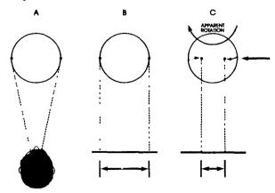
The first step in Terrell's explanation is to draw lines downward (back into the page) from each of the two points on the sphere to a screen direttly below the sphere Figure B is a side view showing the two points, the lines that we have drawn downward, and the screen (If vou hold this book directly in front of you, your eyes are in the same position relative to the dotted lines as the eyes drawn in Figure A)
