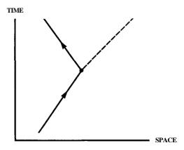
Starting at the bottom, an electron moves through space with a certain velocity. At the point in space and time indicated by the dot, it emits a photon. The photon flys off at the speed of light to the right and the electron, its momentum affected by the emission of the photon, alters course and moves off more slowly to the left.
